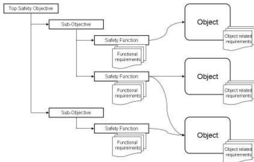
Figure 1 Structure breakdown of functional safety objectives
