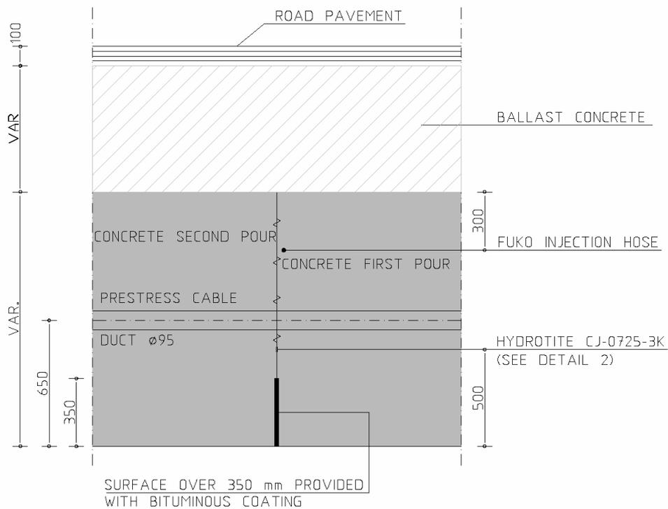
Figure 10: segment joint with crack inducer (bituminous coating) and injection hose
