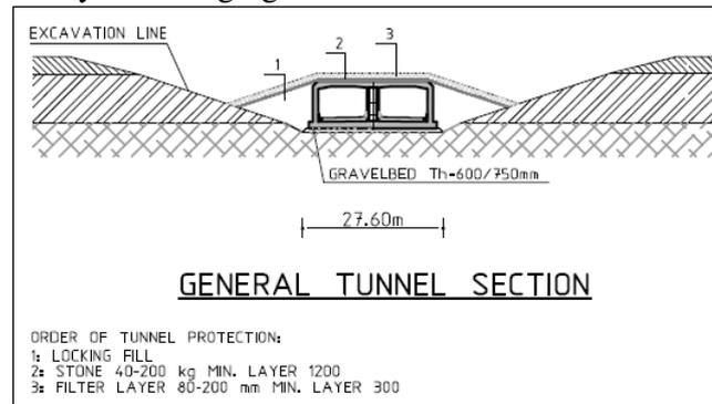
Figure 3: tunnel section
