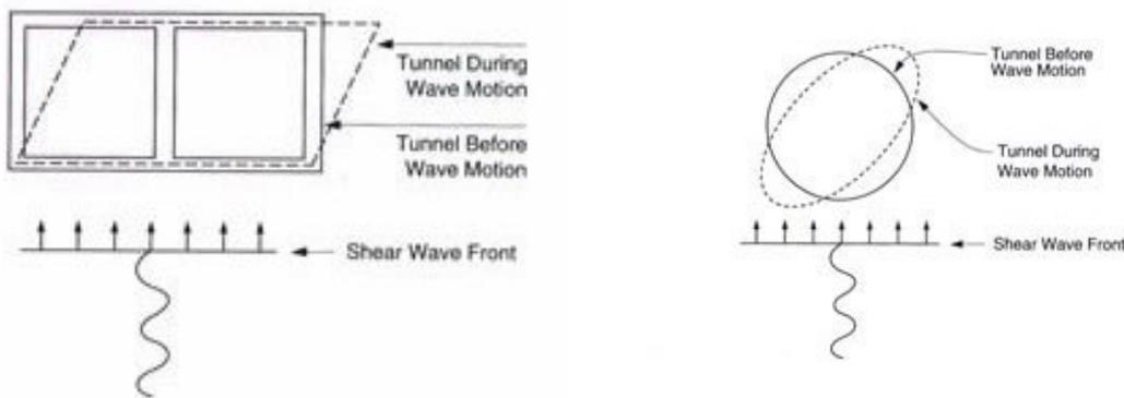
*Racking (rectangular structure) and Ovaling (circular structure): distortion of a transverse cross-sectional geometry due to local soil deformations*
