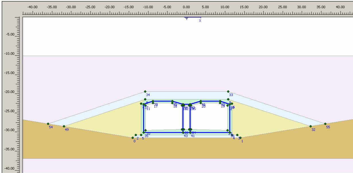
Figure 7: An example of the tunnel profile as modelled in PLAXIS
