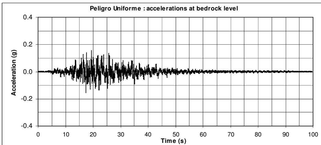
Figure 6: Representative input signal for SHAKE analysis
