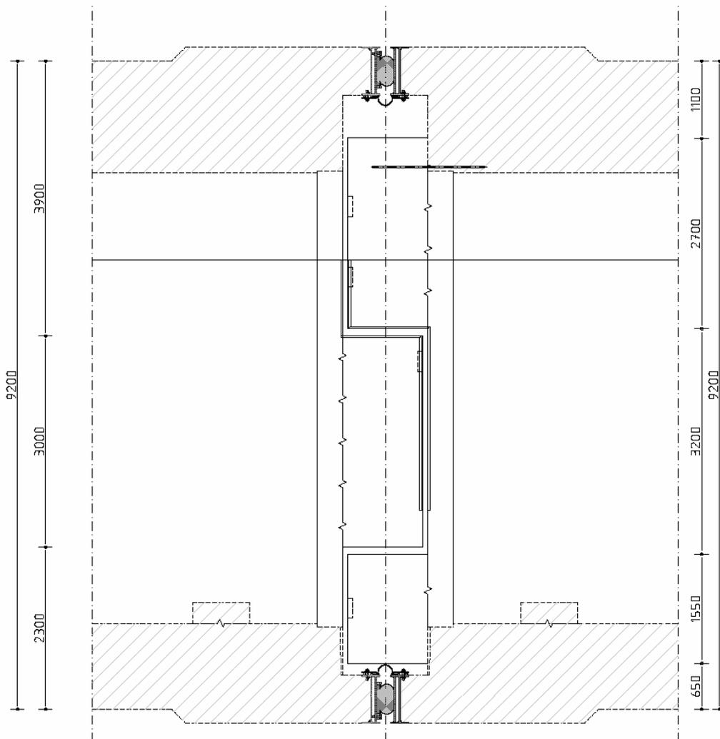
Figure 9: immersion joint with shear keys in the wall
