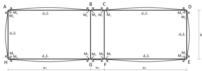
Fig. 10 Tunnel deformation due to thermal distribution in tunnel sections
