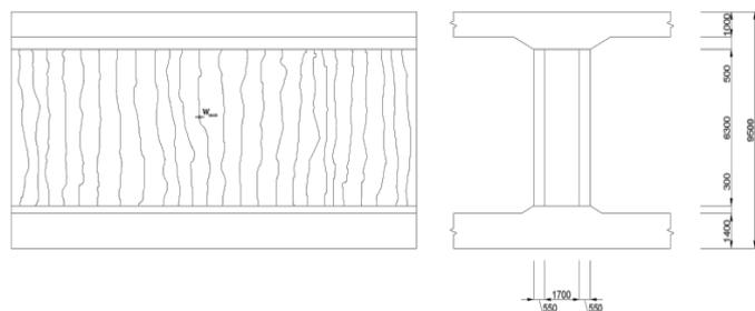
Fig. 9 Cracking due to difference in average temperatures of slabs and edge restraint
