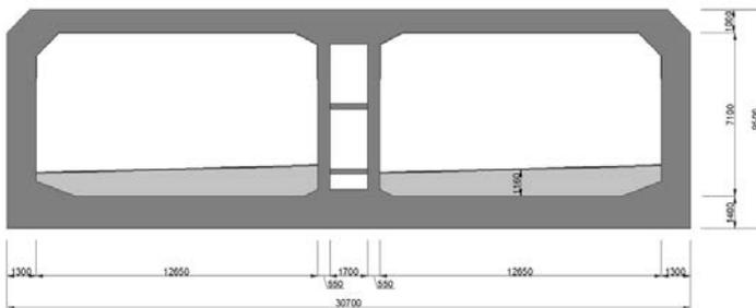
**Fig. 3** A preliminary design of the Orlovsky Tunnel cross-section
