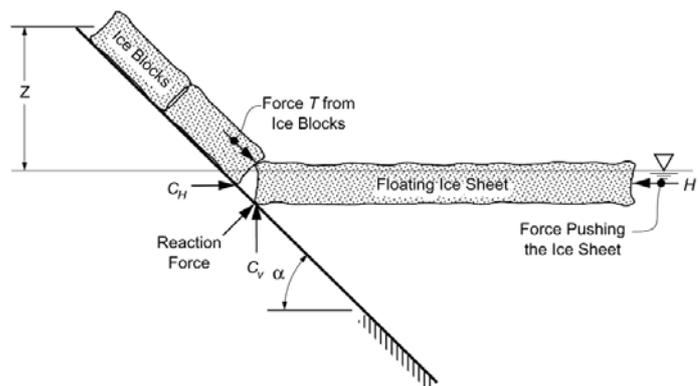
**Fig. 7** Vertical ice loads on sloped embankment (US Army Corps of Engineers, 2002)
