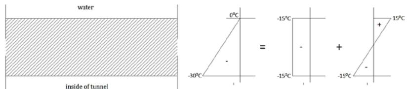
Fig. 9 Temperature distribution in tunnel sections
