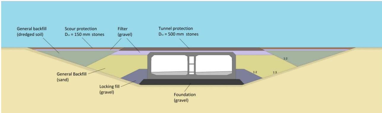
**Fig. 6** Backfill and tunnel protection (inspired by Lunniss & Baber, 2013)
