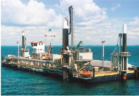
Fig. 11 Scragging Pontoon
